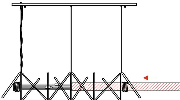
**6** - Put the metal box (ø60 with 40mm) in the same place as the beginning. Conclude with the metal piece .
