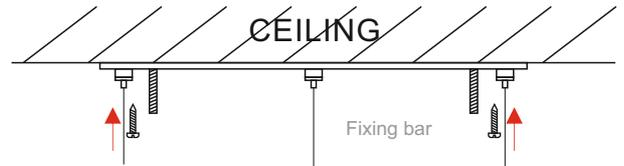
**3** - Connect the electrical wires; Fix the base with the metal buttons and adjust the steel cables with the desired length;
