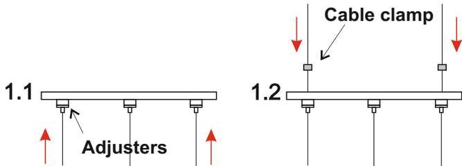
**2** - Fix the fixing bar to the ceiling.
